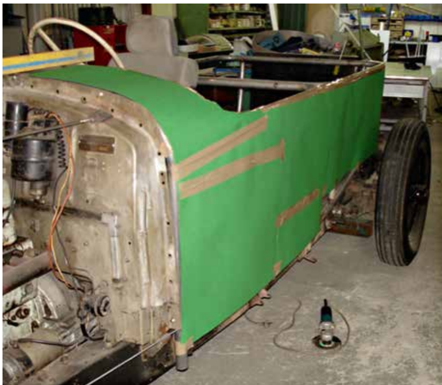
Notice use of the MK VI firewall and scuttle shape.
