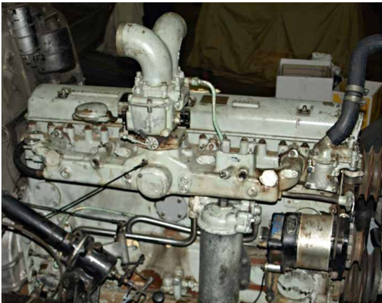
The Rolls-Royce B81 as extracted from its hibernation box, but with Mk VI generator fitted.
