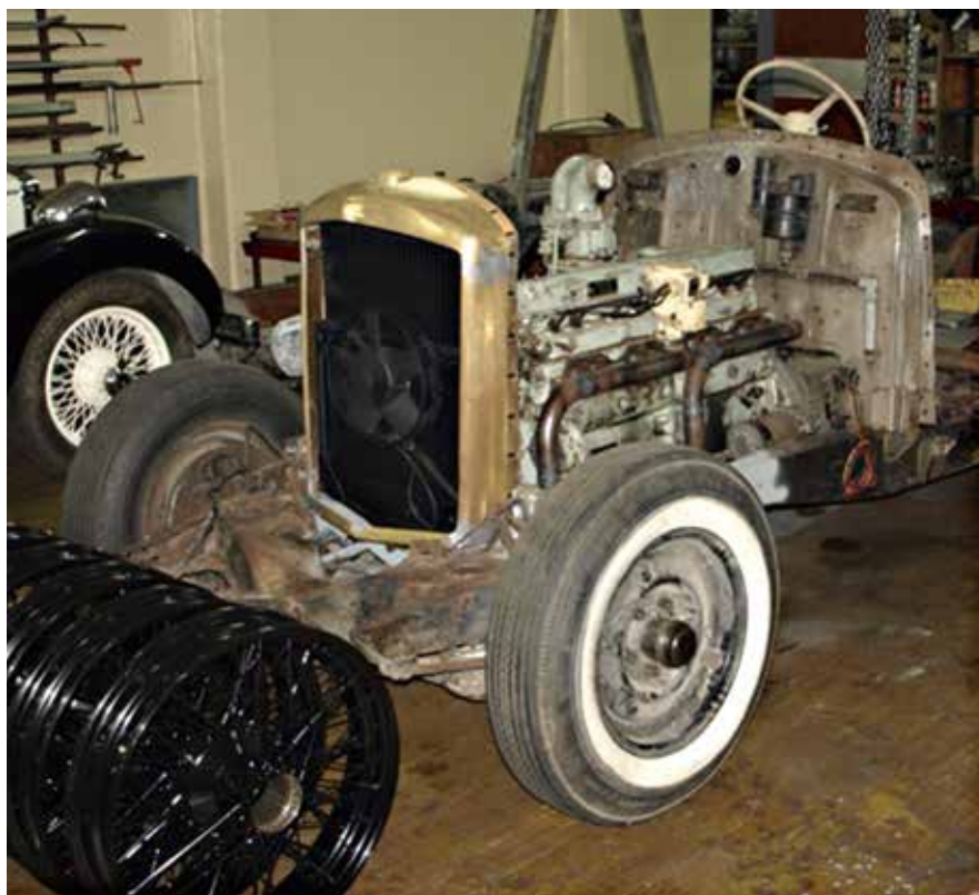
8 Cylinder engine installed and connected up—notice the standard Mk VI wheels and the new black 21 inch wheels ready for tyres.
