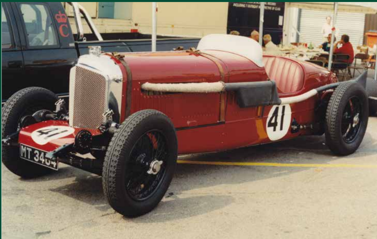
Old Number One as rebodied for Ed Hubbard, improbably finished in red. The body is wrong, because it was made from an offside photograph only so they made the cutaway the same on both sides; the 1932 photograph above shows that the cutaways were asymmetric. The radiator is also wrong. This is something I often see with restoration work. All too often things are 95% right and 100% wrong. The finish in 1932 was grey. The pick-up truck with the 'C' coronet was Hubbard's after some fandango he'd set up to drive the then Prince Charles at Brands Hatch in 1988 in a fund-raiser
